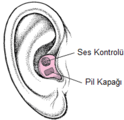
Şekil 9. Kanal İçi İşitme Cihazı ( https://www.msdmanuals.com/en-jp/home/multimedia/figure/hearing-aids-amplifying-the-sound )
