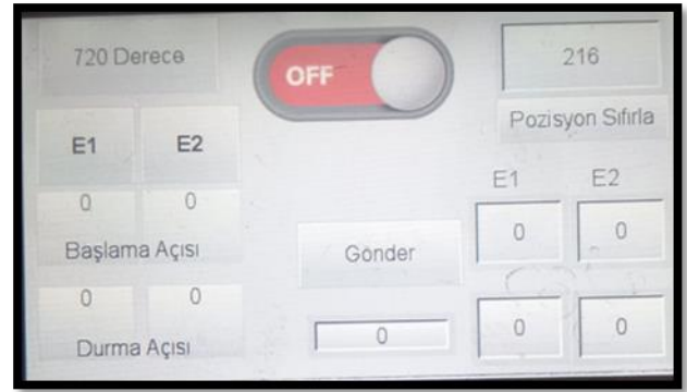
Figure 3: LRF injection system screen
