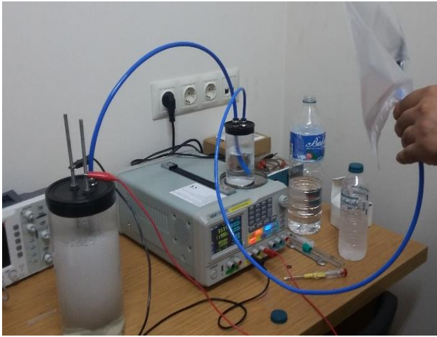
Figure 12. Hydrogen production system.
